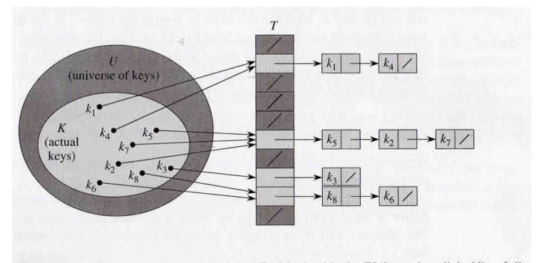
**Figure 11.3** Collision resolution by chaining. Each hash-table slot T[j] contains a linked list of all the keys whose hash value is j. For example,  $h(k_1) = h(k_4)$  and  $h(k_5) = h(k_2) = h(k_7)$ .
