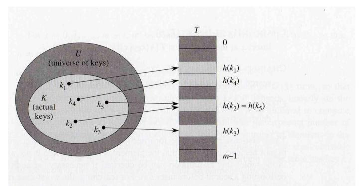
**Figure 11.2** Using a hash function h to map keys to hash-table slots. Keys  $k_2$  and  $k_5$  map to the same slot, so they collide.
